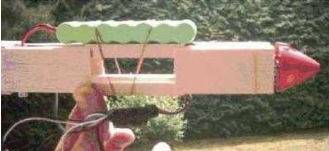
Connected with 10 plates 80x35mm, with obviously wrong fibre direction.
