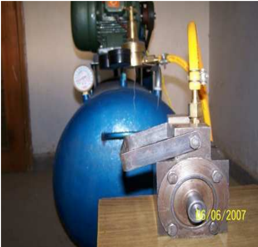
Fig. 4 Compressed Air Turbine –Model under Test
