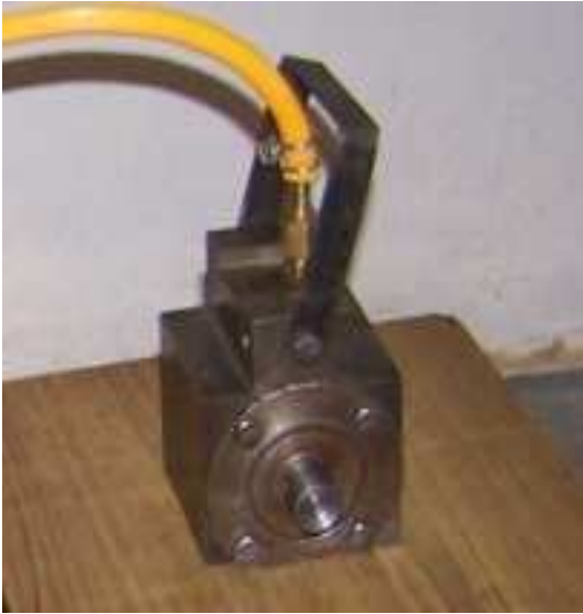
Fig. 3 Compressed Air Turbine –Working Model
