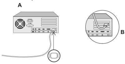
3. Connect the power cord to the power port on the back of your monitor if the power cord supplied is not attached to the monitor. Then insert the plug into a properly grounded electrical outlet.
