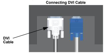
4. Connect the DVI connector at the other end of the signal cable to the DVI port located on the back of the graphics adapter. See picture below.
