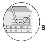
3. Connect the power cord to the power port on the back of your monitor if the power cord supplied is not attached to the monitor. Then insert the plug into a properly grounded electrical outlet.
