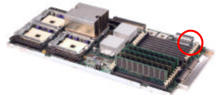
SMP Expansion Module with cover off
