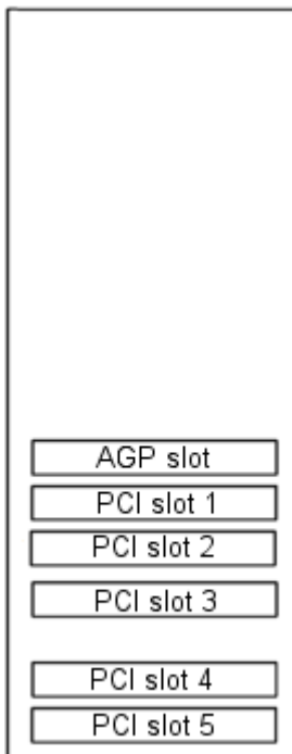
PCI 1-PCI 5: Bus 3, 33MHz, 32-bit, 5v, full-length, PCI
