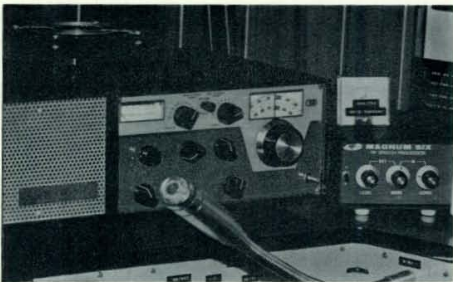
An exciter grid current meter sits atop the Magnum Six RF Speech Processor. The muffin-type cooling fan can be seen on the T-4XB.
