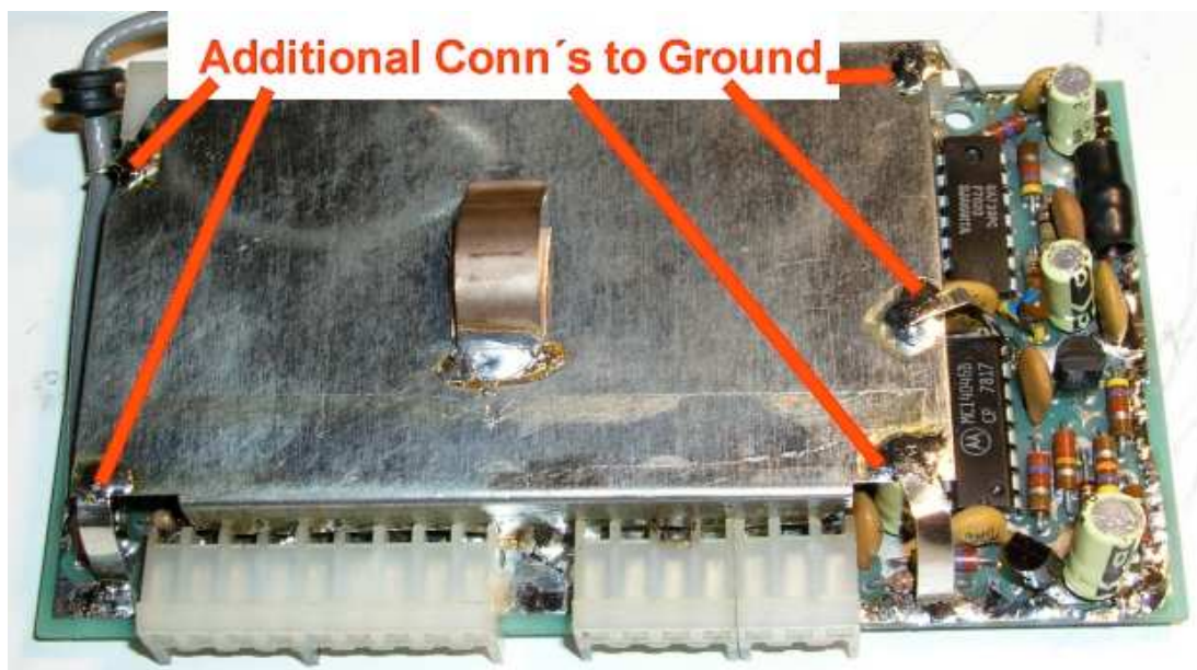
Picture 11: Shielding used as additional ground-layer
