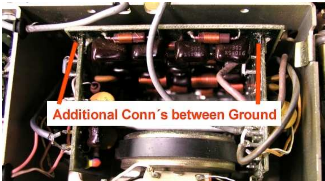
Picture 4: Additional groundconnections in the highpassmodule
