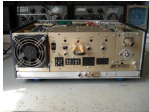
TR7 with rear side extension installed
