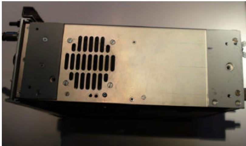
Spacer strips at the left side of TR7
