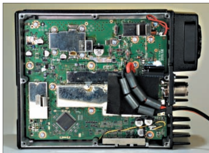
● Inside view of main chassis, showing the large ferrite feed-through bead filters on the d.c. power supply input.
