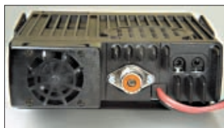
● Rear view of the transceiver, showing centrally-placed antenna socket.
