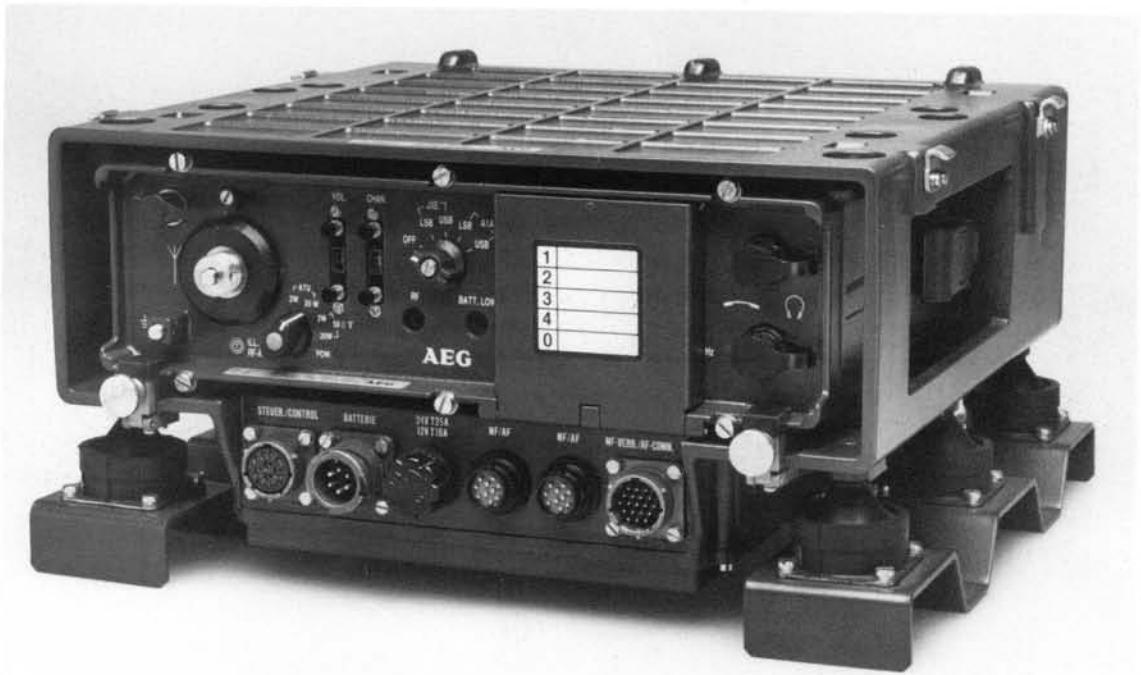
Fig. 2 Basic unit in Vehicle Mount FH 6865/24
