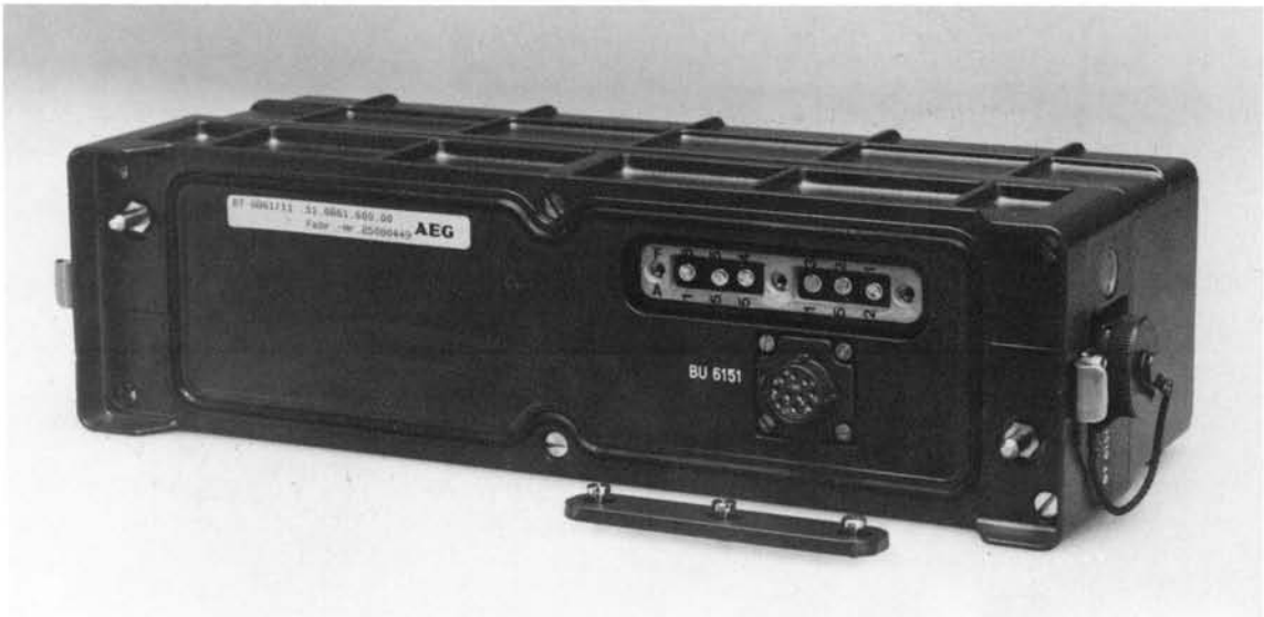
Fig. 35 Battery pack front head BT 6861/11 with removed fuse cover
