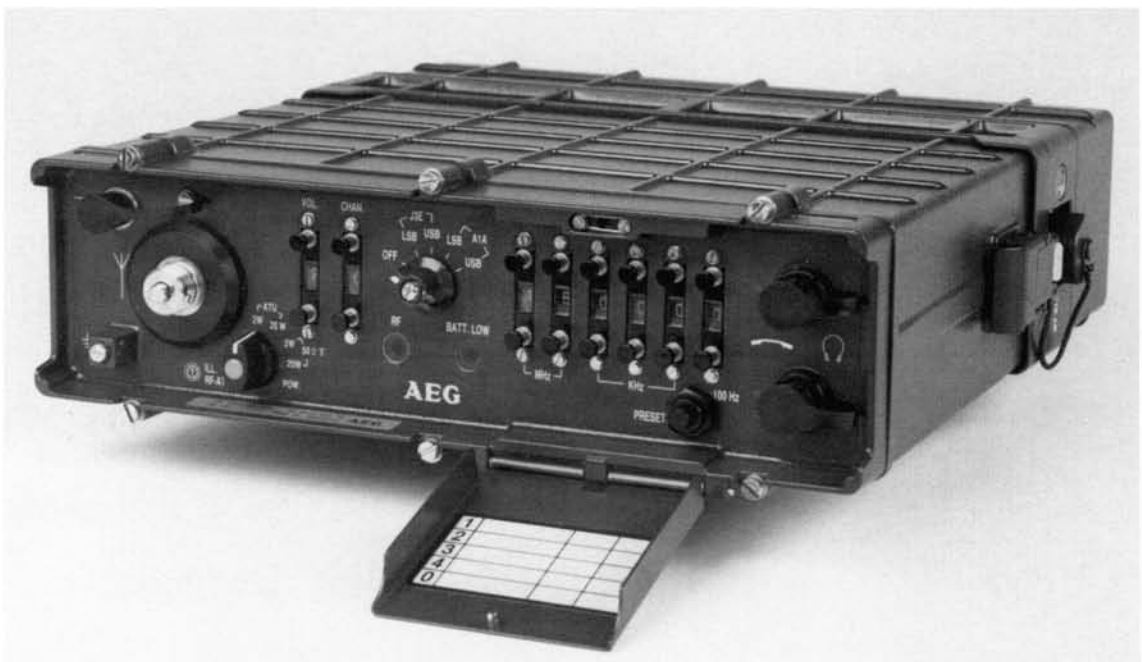
Fig. 1 Basic unit with standard fronthead and Battery pack BT 6861/11
