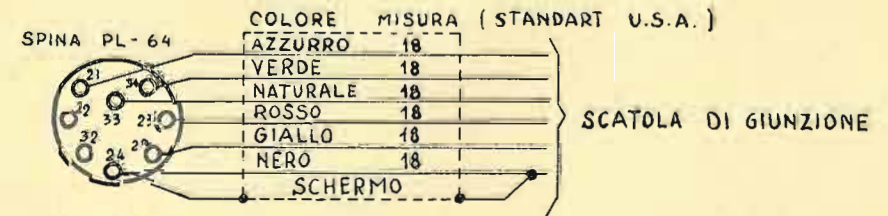
Fig. 19 — Cablaggio dei cavi CD-359, CD-410, CD-471, CD-603, CD-1087, CD-1171.
