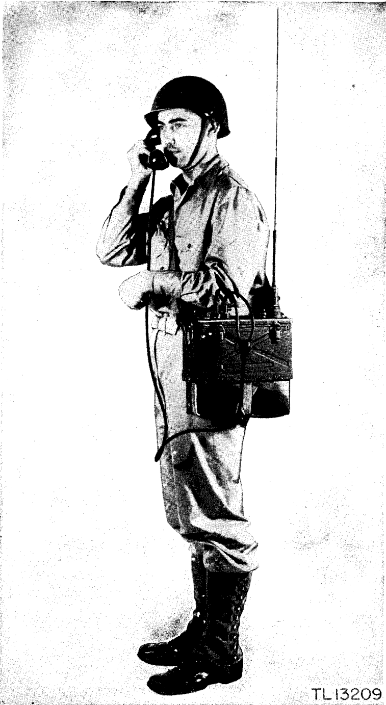
Figure 19. Radio Set SCR-300-A, lightweight installation.
