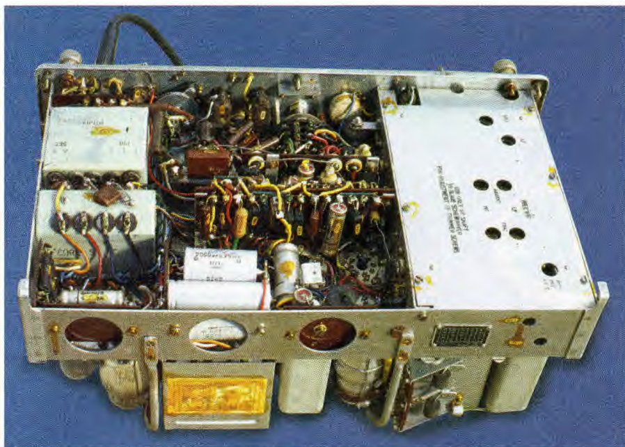
Under chassis view showing the shielded RF section compartment and the crowded wiring.
