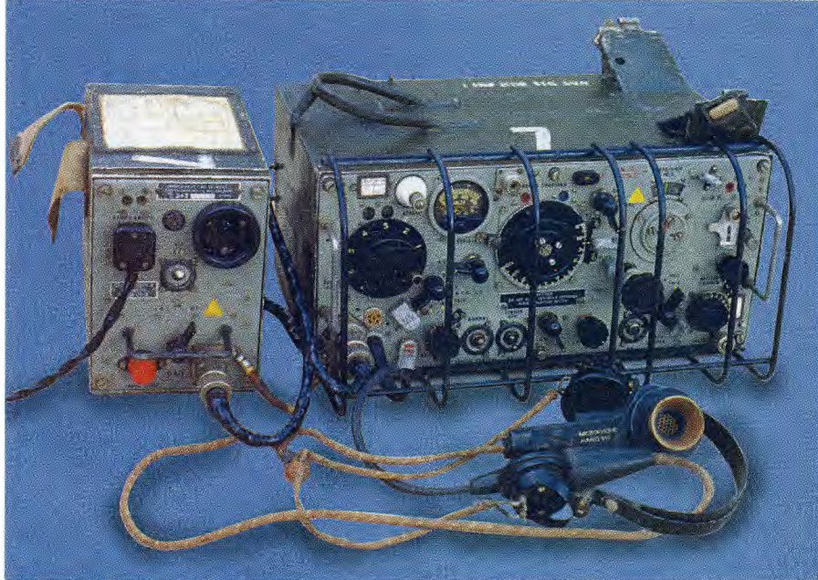
This photo shows the WS122 ready for service with power supply and ancillaries hooked-up. The protective grille at the front made it difficult to operate and most users discarded these.
