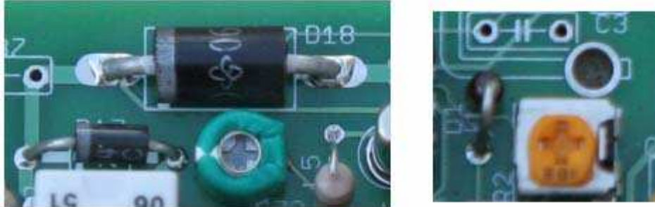
Illustration 1: D-17 and D-18 Installation (N7VE Photo)
