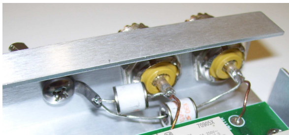
Detail 3. Gas discharge tube mounting
