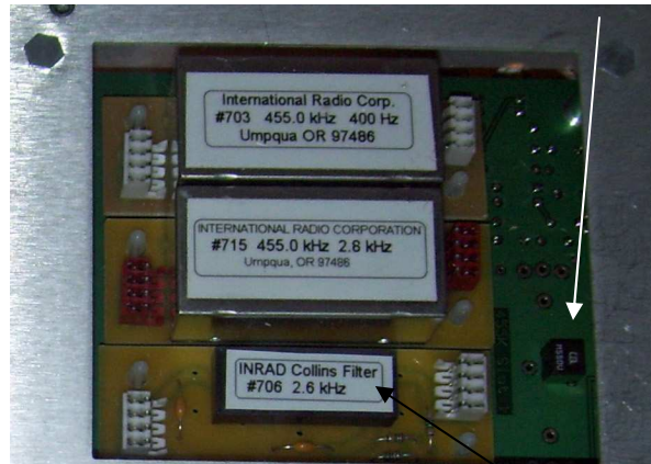
455kHz IF: Collins mechanical filter in slot 2
