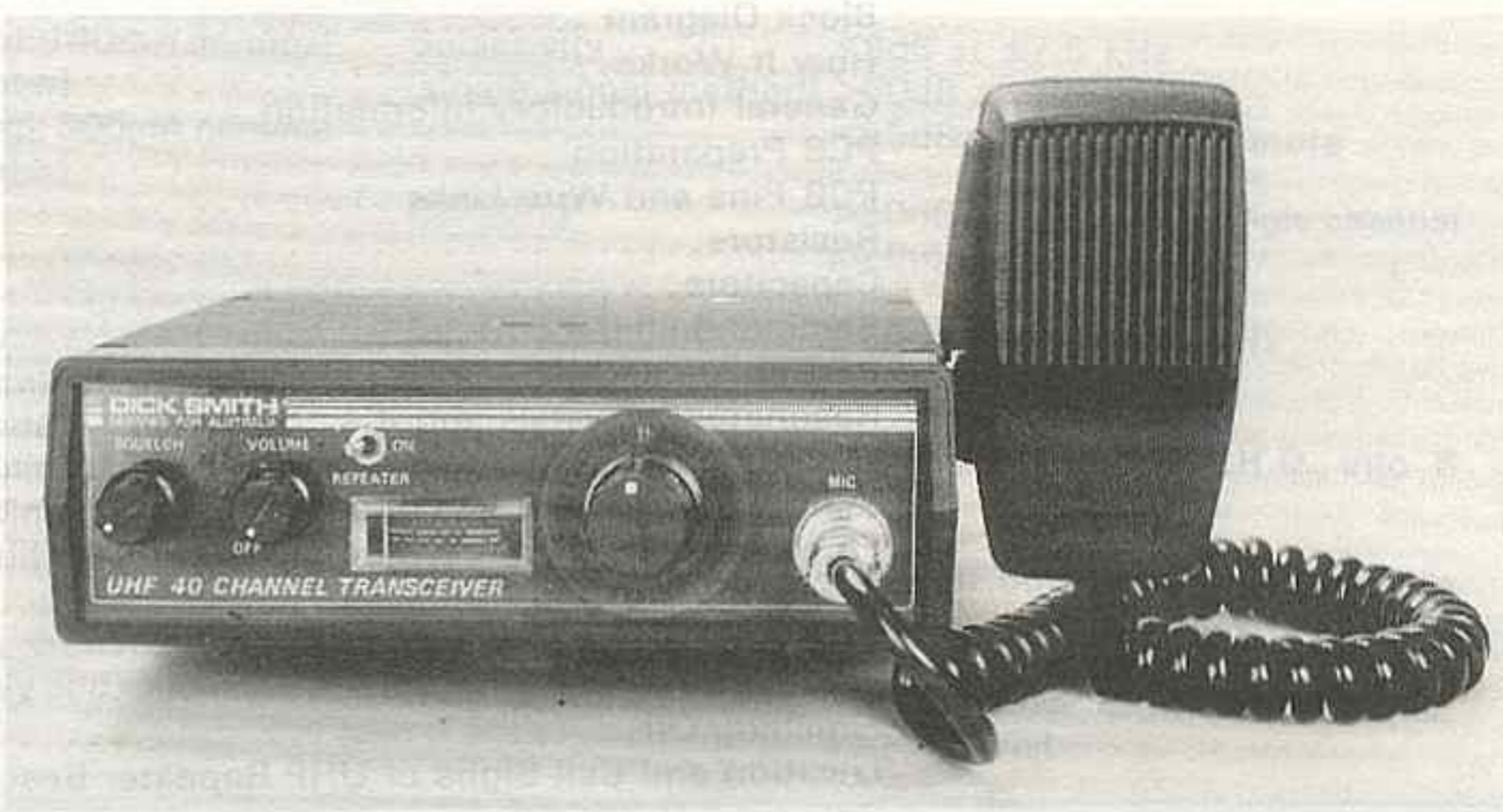
This photograph shows the completed kit (including the optional S-meter and repeater switch). Notice how the microphone plug is mounted on the right hand side of the unit – a feature many commercial units lack.
