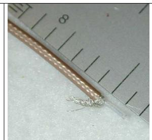
Solder the coaxial cable center conductor to the ungrounded pad at J903.
