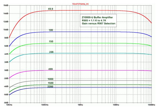
If it is necessary to operate the Z10000-U with less than -4.2 dB gain, C901 can be reduced, or in the event extreme gain reductions are required, R905 may also be reduced to provide an RC voltage divider at the amplifier's input. Although this will introduce some RC frequency shaping in the Z10000-U's frequency response, the passband tilt will be insignificant when used with a Z90 panadapter.
