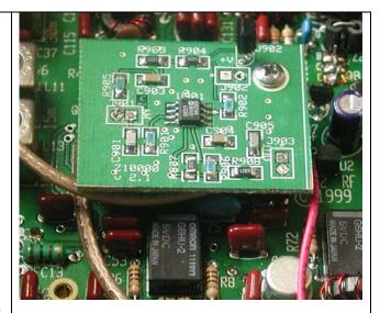
center conductor to the non-ground side of J901. Solder the coaxial cable shield to the grounded pad at J901, trimming its length if necessary to ensure that the braid does not cause a short circuit to the input or any other component. Check the center conductor resistance to ground with an ohmmeter. It should read as an open circuit.
