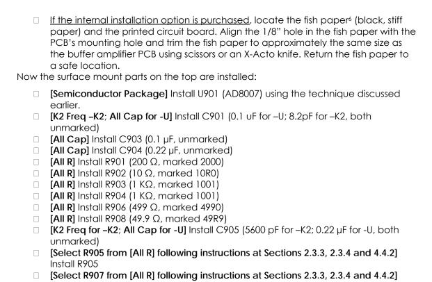
Flip the board upside down and install the remaining surface mount components:
