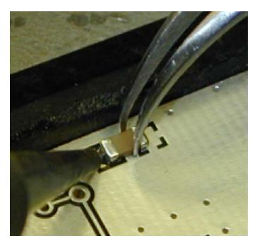
It does not take a large amount of solder to properly attach a surface mount component. A correctly installed part will be flush against the board and have a small filet at the end caps.
