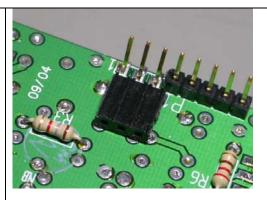
Another view of how the three-pin socket is solder to the modified noise blanker header.
