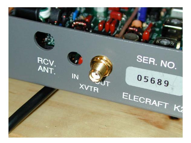
Note that the RCV. ANT. hole is a bit large to properly hold the SMA connector.
