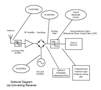
immediately after the first mixer is a crystal filter of perhaps 20 to 25 KHz bandwidth, commonly called a "roofing filter." If the Panadapter is to have maximum utility, it must be connected ahead of the roofing filter.
