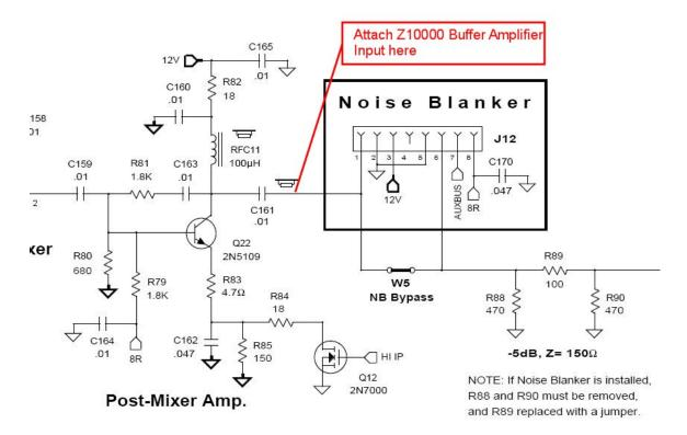
Elecraft has conveniently provided the three connections the Buffer Amplifier needs (signal sample, ground and +12 V) at J12, the noise blanker connection socket, on three consecutive pins, no less. The following sections describe how the Buffer Amplifier is connected and installed, whether the noise blanker board is present or not. The Buffer Amplifier, if installed as described, will not interfere with the noise blanker's operation, should it be installed.
