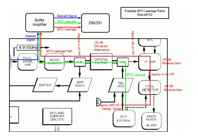
It's not clear which of the two possible paths the culprit is. Considering that the BFO signal is quite strong (I measured nearly 2 volts peak-to-peak at U11), even if it is attenuated 90 dB, it still shows up as a clearly visible signal at the IF pick-off point.
