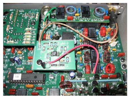
Bob's K2 with the buffer amplifier in place. Note the SMA connector mounting in the space between the 160 meter board and the edge of the back panel.
