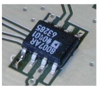
how the PCB was constructed, it may have sufficient solder plating so that additional solder is unnecessary—simply touching the soldering iron to the pin and pad flows enough solder to form a reliable joint. If this isn't possible with your PCB, then apply a <u>small</u> amount of solder to form the joint.
