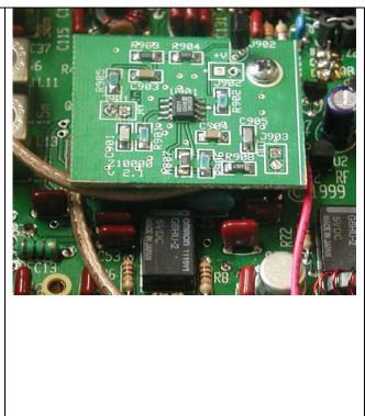
center conductor to the non-ground side of J901. Solder the coaxial cable shield to the grounded pad at J901, trimming its length if necessary to ensure that the braid does not cause a short circuit to the input or any other component. Check the center conductor resistance to ground with an ohmmeter. It should read as an open circuit.
