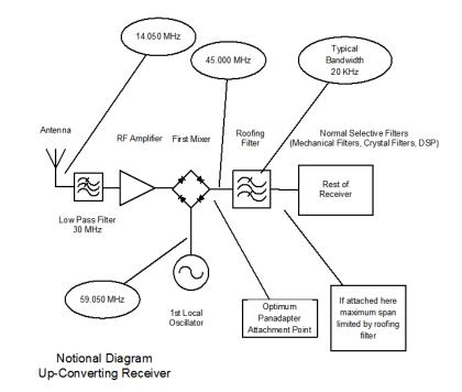
immediately after the first mixer is a crystal filter of perhaps 20 to 25 KHz bandwidth, commonly called a "roofing filter." If the Panadapter is to have maximum utility, it must be connected ahead of the roofing filter.
