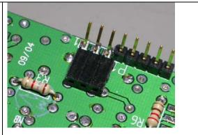
Another view of how the three-pin socket is solder to the modified noise blanker header.
