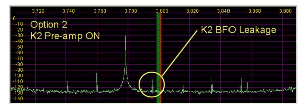
The images show a significant reduction in BFO leakage, on the order of 30 dB.
