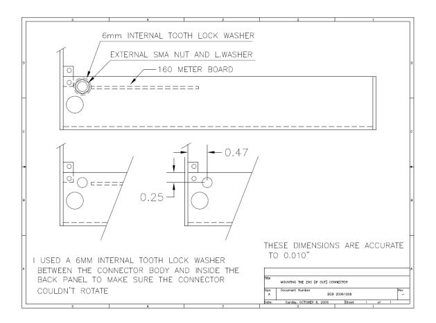
Bob notes that the 6mm ( $\frac{1}{4}$ ") (internal diameter) lock washer just fits in between the "D" chassis bracket and the 160 Meter board so it is necessary to carefully measure the hole's location.
