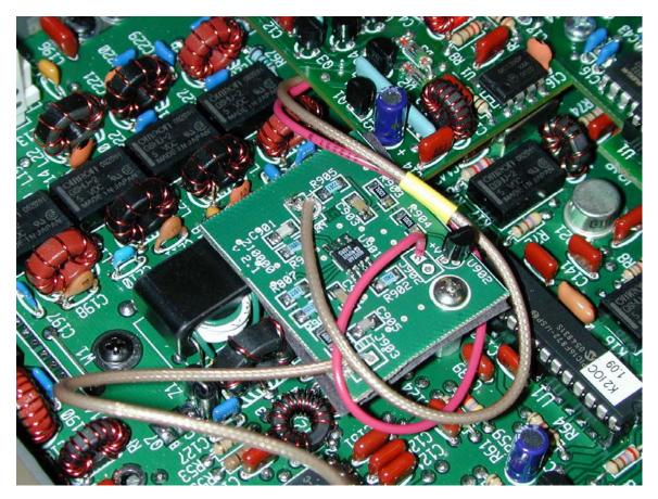
Now that you know where the buffer amplifier will be located, determine where the output SMA connector will be installed.
