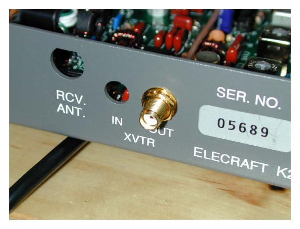
Note that the RCV. ANT. hole is a bit large to properly hold the SMA connector.
