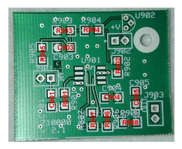
The photograph shows an earlier version of the PCB. Later PCBs correct the silk screen error identifying R907 as R<u>8</u>07, and slightly rearrange other silk screen legends. In addition, production circuit boards may be slightly smaller than in the photographs.
