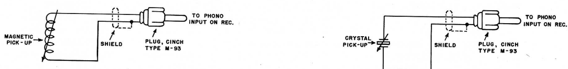
Fig. 4. Wiring diagram, record player connection.
