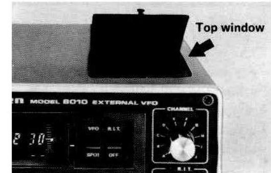
Top window for installing crystals
