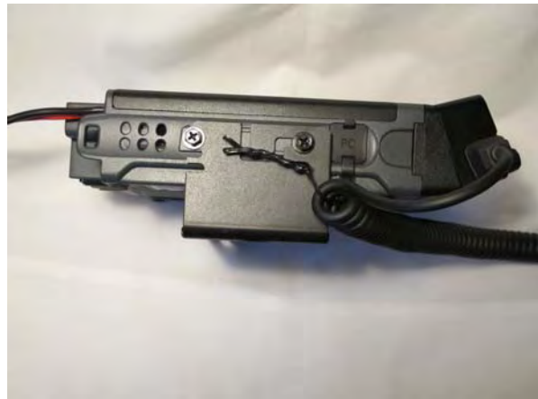
Fig 6 : Makeshift strain relief for mic plug for base station use with mobile bracket used as a stand.
