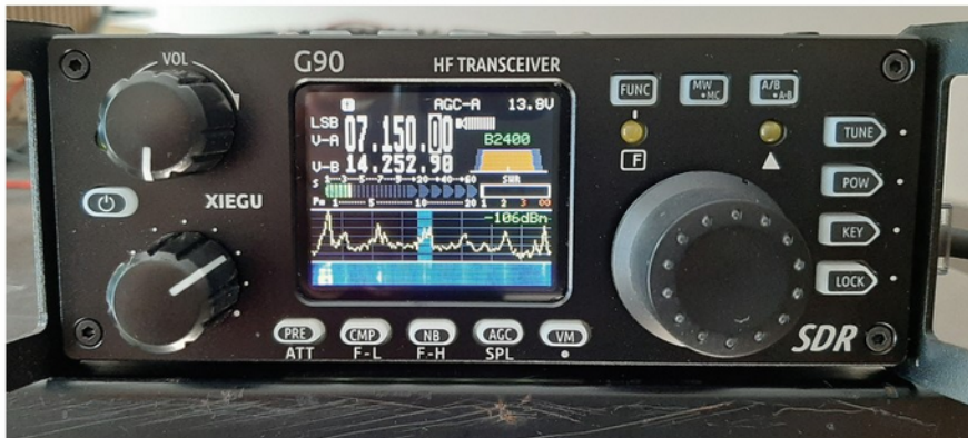
The head unit can be detached from the main body by removing the four hex headed bolts.
