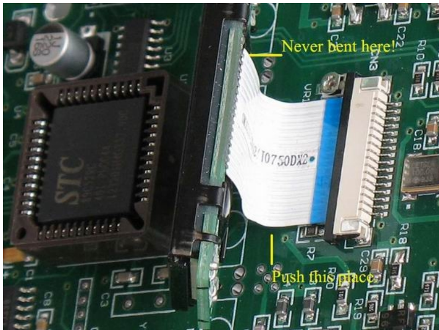
How to insert the LCD Cable
