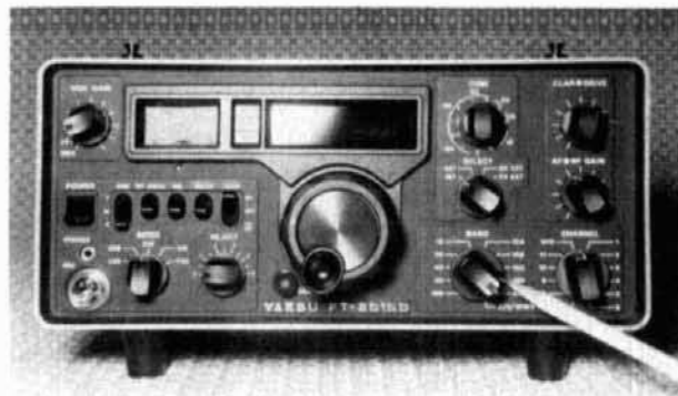
AUX setting of bandswitch used for 30 meters.
