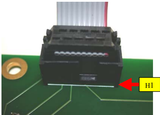
Figure # 10: Insert Female side of Ribbon Cable (P/N 21-30-0034-1) onto H1 making sure it's secure.
