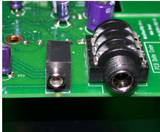
Figure # 1: Make sure J3, J7-J9 (21-00-6616) and J10 (21-00-001) are flush with are PCB before soldering.
