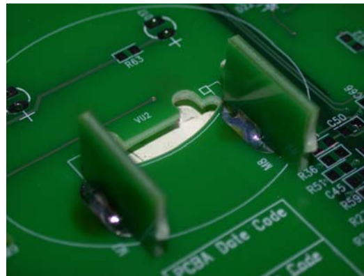
STEP #4: Before soldering, make sure the VU PCB support is straight and flush against the Main PCB.
