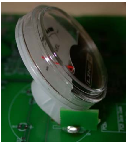
STEP #5: Place one of the VU meters in the silkscreen space on the TOP side of the PCB .
