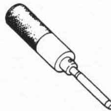
09916-57321 Valve guide installer handle
