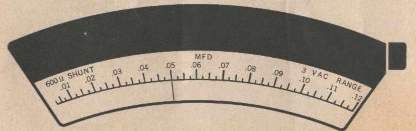
Figure 28—.0025 to .12 mfd Capacity Scale
