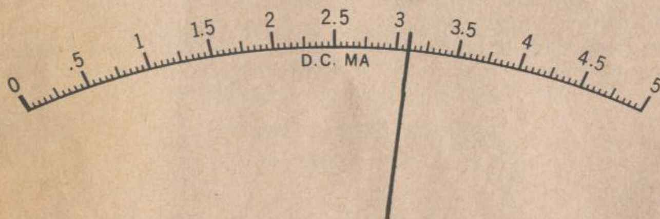
Figure 22—5 MA D.C. Scale
