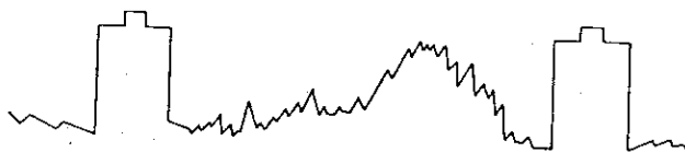
Figure 4 Normal Video and Sync Signal.
