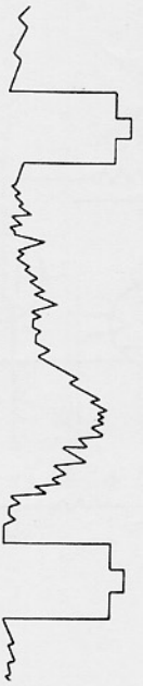
Figure 4 Normal Video and Sync Signal.
