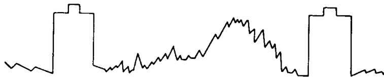
Figure 4 Normal Video and Sync Signal.
