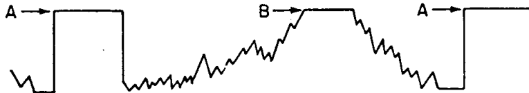
Figure 5 Overloaded or Clipped Video and Sync Signal.
