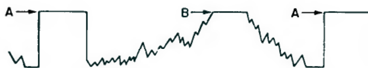
Figure 5 Overloaded or Clipped Video and Sync Signal.
