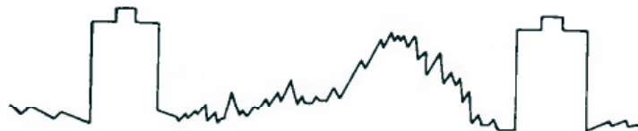
Figure 4 Normal Video and Sync Signal.
