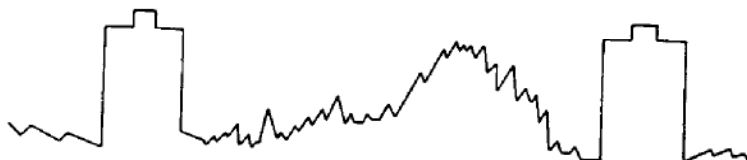
Figure 4—Normal Video and Sync Signal.
