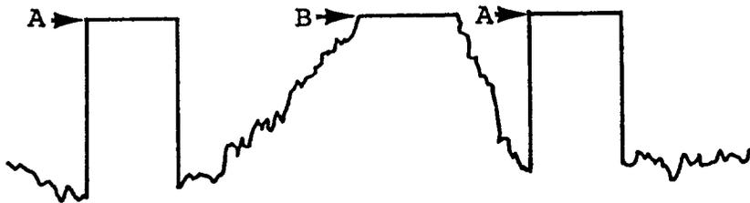
Figure 8. Overloaded or Clipped Video and Sync Signal
