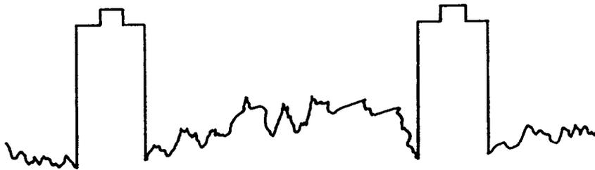
Figure 7. Normal Video and Sync Signal
