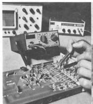
Alpha I is a low cost, professional digital multimeter. Although fully portable, it packs within its case all an engineer needs for day-to-day use.
