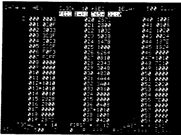
Figure 3.9. Here the unit has been programmed to search for the hex word 1010. It found this word 14 times; first occurrence at memory location 12, and last one at 292. This information is read out at the bottom of the screen. Each occurrence is marked by an asterisk.
