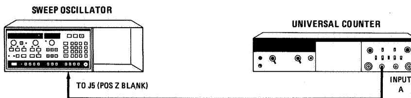
Figure 5-14. 27.8/1 kHz Oscillator Adjustment Setup.
