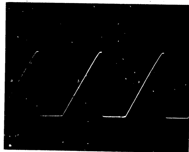
Emitter A1Q1 20 V/div 5 ms/div
