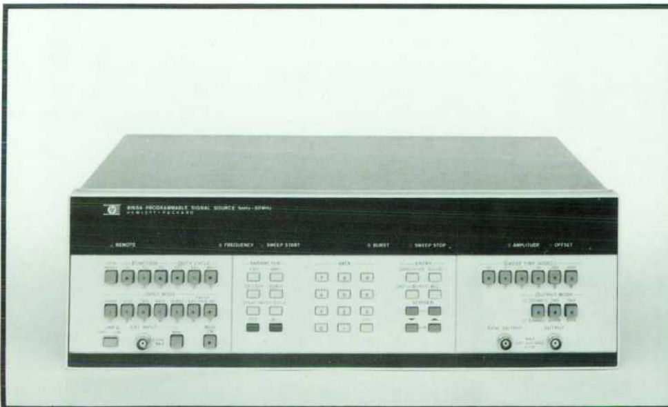
Fig. 1. Model 8165A Programmable Signal Source produces sine, triangle, and square waves in a frequency range of 1 MHz to 50 MHz. It also generates pulses or ramps with 20% or 80% duty cycles in a range of 1 MHz to 19.99 MHz. For stability, the output is phase-locked to a quartz crystal oscillator. HP-IB input/output is standard. An option provides logarithmic sweep and AM.
