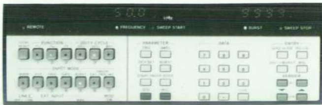
Fig. 7. Mnemonics, indicated on the front panel by framed letters, specify the HP-IB commands necessary to program the corresponding functions.
