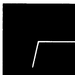
Diode in series with 51Ω
