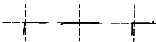
Typ: Normale Diode Hochspann.-Diode Z-Diode 12V Pole: Kathode-Anode Kathode-Anode Kathode-Anode Anschlüsse: (CT-Masse) (CT-Masse) (CT-Masse)
