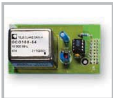
Option H085, a high-stability oscillator with a stability of \pm 5 \times 10^{-9} per day
