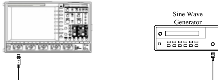
Figure 5-6 : 50Ω Bandwidth Equipment Setup
