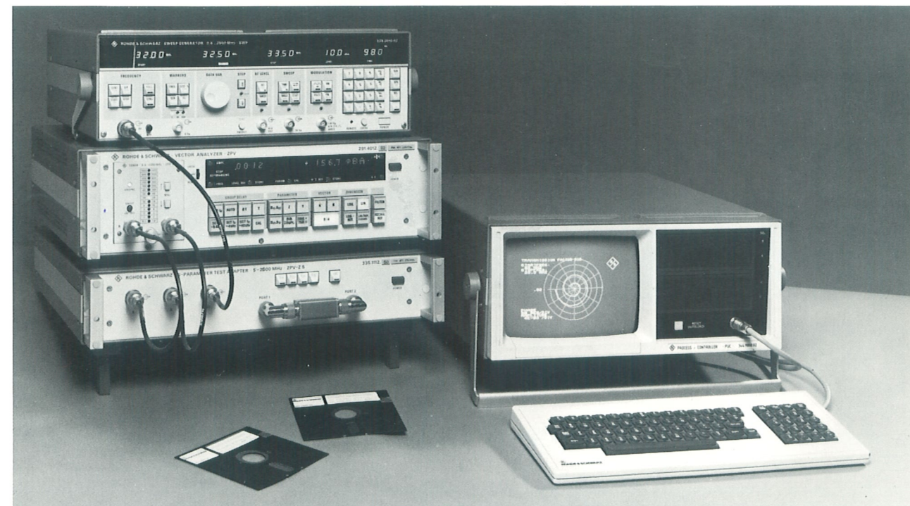
Fig. 2 Automatic network analysis using Vector Analyzer ZPV, S-parameter Test Adapter ZPV-Z5, Sweep Generator SWP and Process Controller PUC
