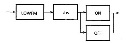
This selects LOWFM when in the automatic acquisition mode. Selecting LOWFM ON while in manual acquisition mode generates an execution error. TRACK ON is disabled if this mode is selected, selecting LOWFM OFF does not reset TRACK to ON.
