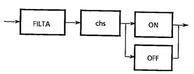
Controls the Channel A low-pass filter. 'ON' switches in the filter and 'OFF' switches it out.
