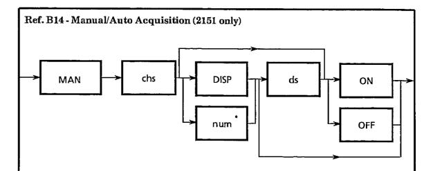
Controls the manual acquisition mode. Two parameters can be specified, these are the value to be entered in the Manual Store and switching Manual Mode ON or OFF. At least one parameter must be entered or a command error is generated.
