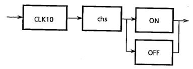
Controls the selection of either the CLK10 reference or the counter reference. 'ON' selects CLK10, 'OFF' selects the counter reference.
