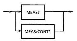
The upper path of this command causes the instrument to abandon any current reading, start a new cycle and place the calculated result into the Output Queue. The lower path is similar, but as soon as the result is read out of the Output Queue a new measurement is taken and placed into the Output Queue.
