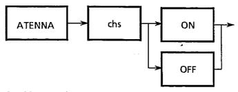
Controls the Channel A x20 attenuator. 'ON' switches in the attenuator and 'OFF' switches it out.
