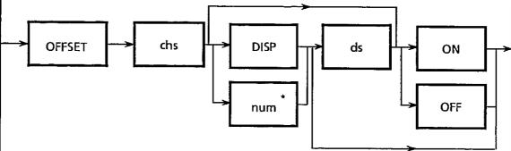
This controls the offset mathematics function. Two parameters can be specified, these are the value to be entered in the offset store (of which there are two sources), and turning the function ON or OFF. If no parameters are specified, then a command error is generated.
