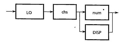
This sets the value of the Local Oscillator to be used when SF 41 is active.
