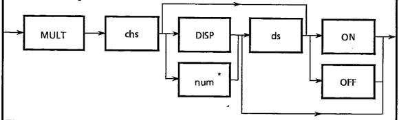
This controls the multiplier mathematics function. Two parameters can be specified, these are the value to be entered in the multiplier store (of which there are two sources), and turning the function ON or OFF. If no parameters are specified, then a command error is generated.
