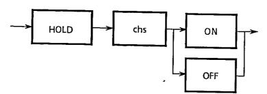
Selects the HOLD mode, suspending repetitive measurements. The reading is held until another is triggered (see \*TRG and MEAS?).
