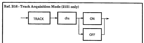
This selects TRACK when in the automatic acquisition mode. Selecting LOWFM ON while in manual acquisition mode generates an execution error. LOWFM ON is disabled if this mode is selected, selecting TRACK OFF does not reset LOWFM to ON.
