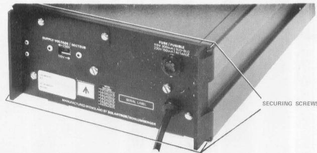
Fig. 4.1. View of Rear Panel, showing location of the 4 securing screws.
