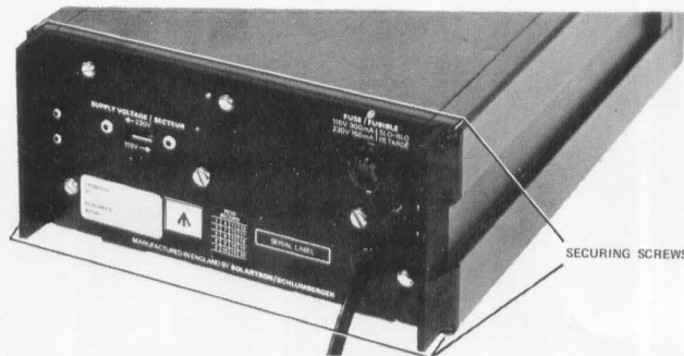
Fig. 4.1. View of Rear Panel, showing location of the 4 securing screws.
