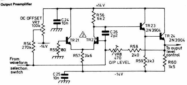
The selected waveform passes to the preamplifier. TR21 and TR22 form a long tailed pair and are in thermal contact with each other to reduce dc drift. TR23 and TR24 are two cascaded emitter followers; feedback is via R58 and VR8. VR8 sets the preamplifier gain and is adjusted to give 10V peak to peak into 50 ohms at the 50 ohms output.
