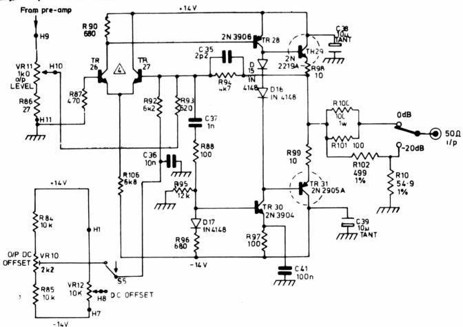
TR26 and TR27 form a long tailed pair and are in thermal contact with each other to reduce dc drift. TR28 is the driver transistor and TR30 its collector load. TR29 and TR31 are complementary output transistors and diodes D15 and D16 provide their bias. C37 and R88 are feedforward compensation components to increase the
