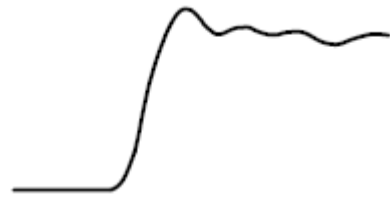
Long ground lead
